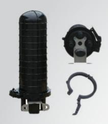
GPJM3-RS provide with four fiber cable in-out ports (3 round ports, 1 elliptical port), it can be used in aerial and underground application, it is made from quality engineering plastic, the cover and the base are filled with silicon rubber and sealed with hoop, then entry ports are sealed with thread parts, it can be opened after sealing and can be reused without changing sealing material.
